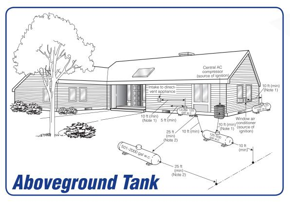
The location of the container is important. Specific rules about the placement of liquid containers can be found in the National Fire Protection Association's (NFPA) 58. There are standards for ASME aboveground containers, ASME underground containers, and DOT cylinders.
