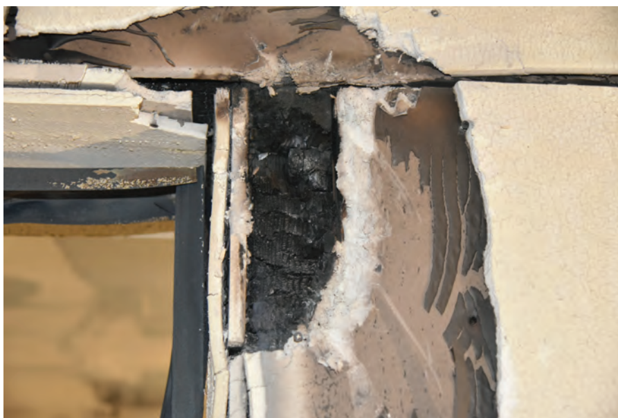
Glulam beam-to-column connection as part of an assembly fire test.
