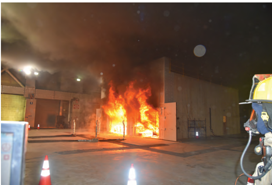
Mass timber construction fire test.
