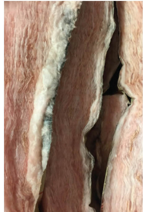
Kraft-paper-backed fiberglass. Insulation is a Class II vapor retarder.
