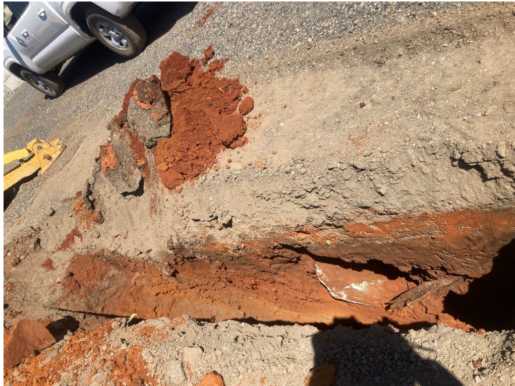
Photo No. 3 – Grey fill layer over reddish brown alluvium
