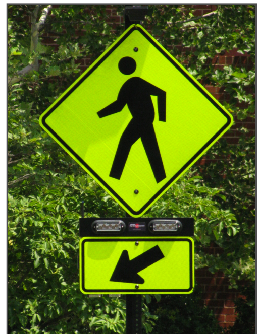
A Rectangular Rapid-Flashing Beacon (RRFB). Source: Carol Kachadoorian (2012)
