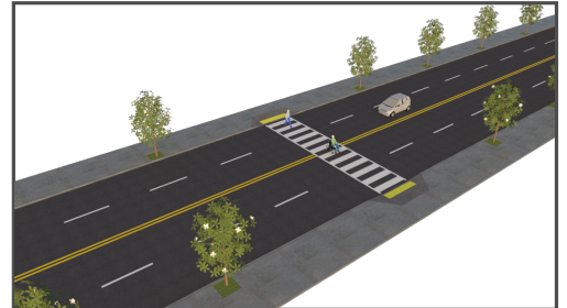
This rendering shows a four-lane road with a midblock crosswalk before a road diet. Federal Highway Administration.
