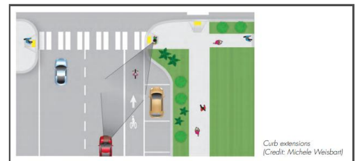
Curb extensions improving the ability of pedestrians and motorists to see each other. Living Streets Page 7-13
