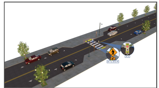
The enhancements shown in this rendering of a midblock crosswalk include high-visibility markings, curb extensions, in-street pedestrian crossing signs, lighting, and warning signs. Federal Highway Administration.
