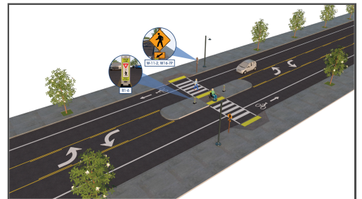
This rendering shows how a road diet on a street that was previously four lanes can create space for features like bicycle lanes and a pedestrian refuge island. Federal Highway Administration.
