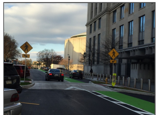
Raised pedestrian crossing with curb extensions at a midblock location on a one-way street with a bike lane. Pennsylvania Department of Transportation.
