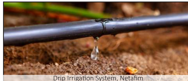
Drip Irrigation System, Netafim
