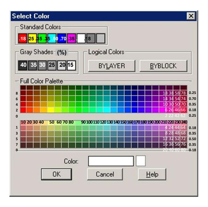
The first digit(s) of the color number represent the percent shading, while the last digit represents the pen weight associated with the corresponding pen weights of colors 1 through 9 above.
