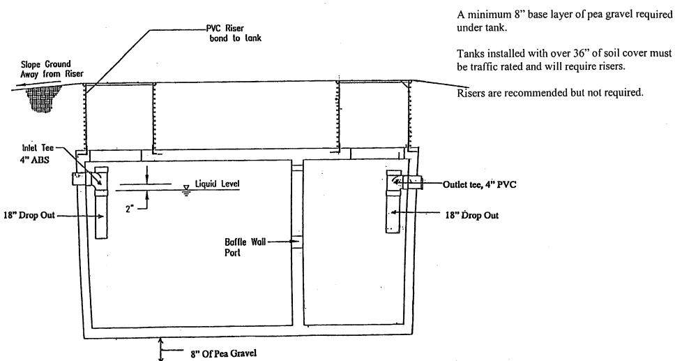
Building Sewer Must Be 4 " ABS with a clean out.
