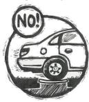
**Don't** drive over your tank or any buried components in your system, unless it's been equipped with a special traffic lid. If the system is subject to possible traffic, put up a barricade or a row of shrubs.
